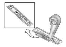
**P (Park):** This position locks the front wheels. It is the best position to use when starting the engine because the vehicle cannot move easily.
